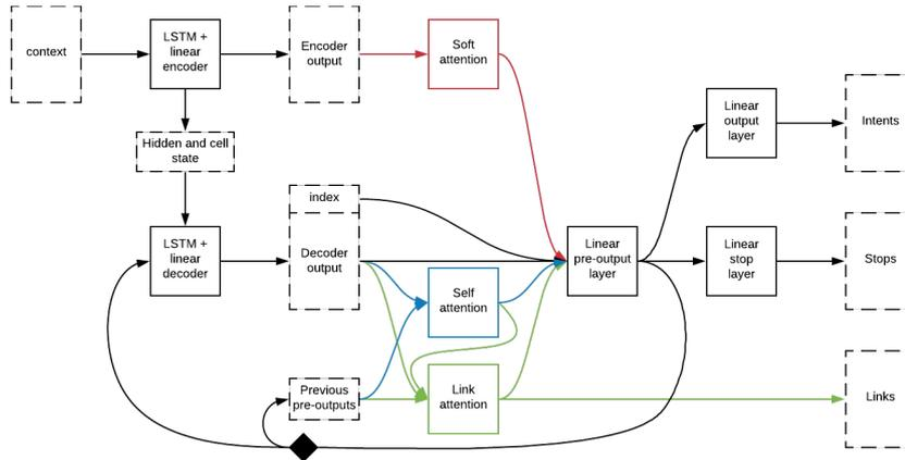
FIGURE 4.4: Block diagram of the recurrent architectures.
