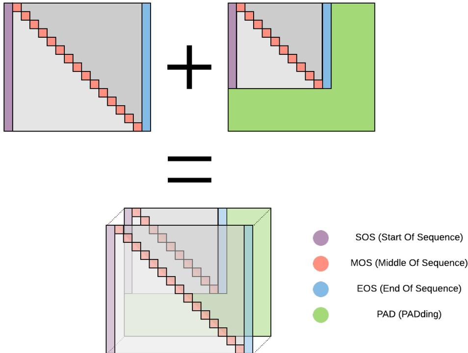
FIGURE 2.2: Diagram of a batch of 2 samples encoded using the 6 values NO EDGE (0) and EDGE (1) for the adjacency, SOS, MOS, EOS, and PAD.
