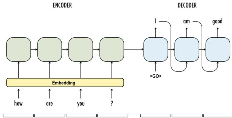
FIGURE 4.3: Example of a sequence to sequence RNN, figure from [24].
