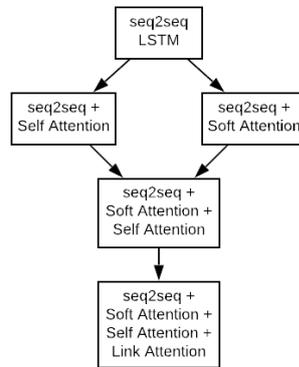
FIGURE 4.5: Hierarchy of the tested recurrent architecture variants
