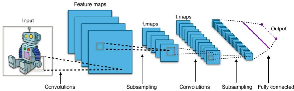
FIGURE 1.4: Example of CNN architecture. From Wikipedia.
