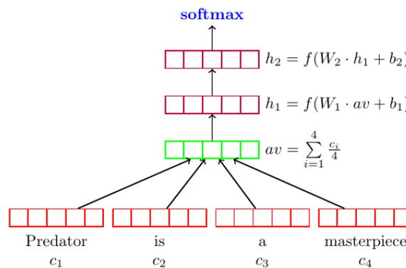
FIGURE 1.7: Example of DAN, Figure 1 from [23].
