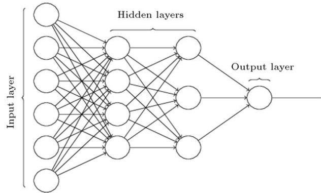
FIGURE 1.3: Multi-layer perceptron architecture. From [https://www.researchgate.net/profile/Ayhan\\_Erdem2/publication/319309006](https://www.researchgate.net/profile/Ayhan_Erdem2/publication/319309006).
