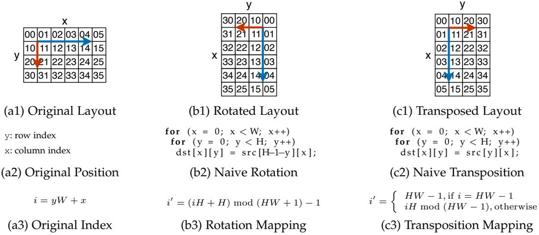
Fig. 1. Matrix Rotation and Transposition: data layout transformation examples, naive codes and linear mappings for  $H \times W$  matrices
