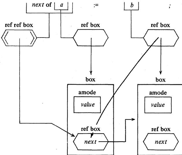
The result is that we have chained the **box** referred to by *a* to the **box** referred to by *b* via the *next of* field of the **box** *a*.
