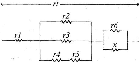
It is required to find the value of  $x$  such that the resistance of the whole network shall be  $rt$ . Here is a program to do it:
