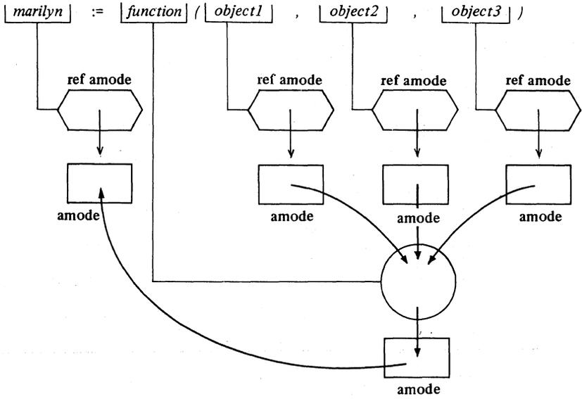
Again, the LHS and the RHS are elaborated collaterally, as are the three actual-parameters *object1*, *object2* and *object3* on the RHS, by virtue of the commas between the formal-parameters in the routine.
