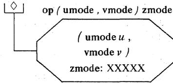
In contrast to procedures, an operator can only be defined to yield a routine and not to refer to one. Consequently, the uncontracted forms (as in E5) are rarely of practical use, and we shall never write one again.
