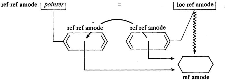
This is essentially the same as E3. The generator `loc ref amode` generates a name on the stack. Such a `ref amode` on the stack may, by assignation to `pointer`, become an instance of a name referring to an `amode` object on the stack. In this way, “indirect addressing” is another fruit of the general concept of an identifier-declaration.
