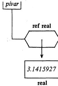
To *pivar* any other value can be assigned, *pivar* being a variable.
