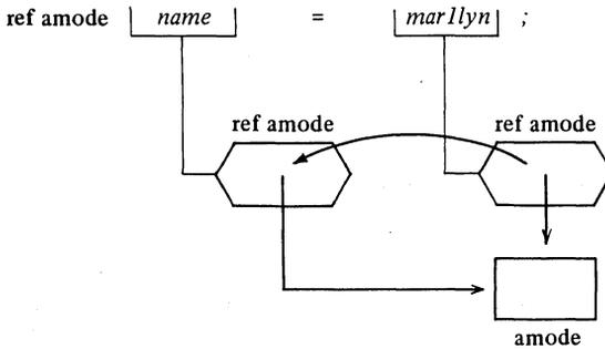
The result of the elaboration of E2 is that we have got two different identifiers, *name* and *marllyn*, yielding different instances of the same name and consequently referring to the same internal **amode** object.
