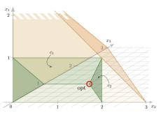
**Fig. 2:** Feasible region (green), global capacity constraint (orange) and solution profile of Example 1.
