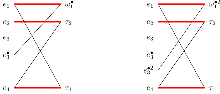
Figure 17: An example with c_f^- > c_f : another variation on the clutch. The previous mode determines \omega_2^{\bullet 2} , hence \omega_2^{\bullet} is no longer a dependent variable when entering the new mode. Maximal cardinality matchings for N = 1 (left) and N = 2 (right) are shown. Subsequently applying the Dulmage-Mendelsohn decomposition on the left-hand graph returns \beta_\Sigma = \mathcal{G}_F , hence Line 6 of Algorithm 10 returns H = \emptyset . No equation of the new mode is satisfied at the first instant and we move to the next instant. The same holds for the right-hand graph.
