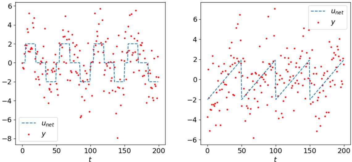
Figure 4: 2 types of simulated periodic signal ( $u_{net}$ ). Examples of  $y = u_{net} + \epsilon$  with  $\epsilon \sim \mathcal{N}(0, 4)$  are shown. Left: Piece-wise constant; Right: Piece-wise linear.
