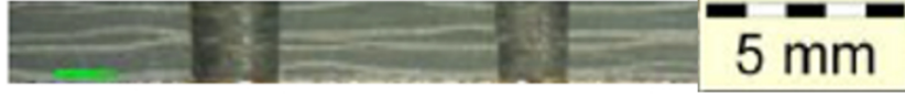
FIG. 3. Cross-sectional view of a perforated plate with R_{\text{neck}} = 0.9 mm. Note that this view does not intersect with both of the perforations axes.
