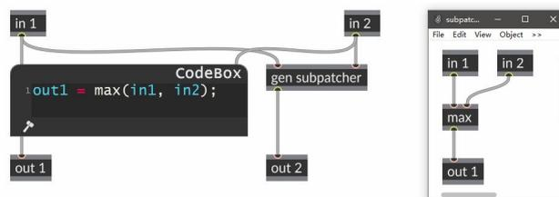
Figure 3 Gen example: sub-patcher and code block
