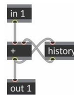
Figure 4 Gen example: a feedback with one-sample delay
