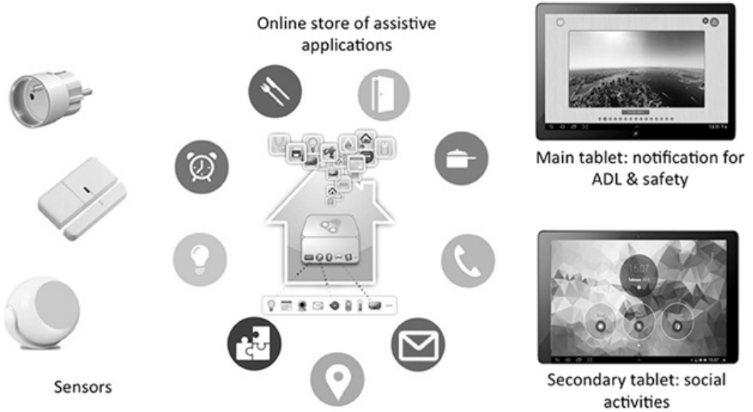
Figure 1. Content of the HomeAssist platform: A set of sensors, an online catalog of assistive applications and two touchscreen tablets
