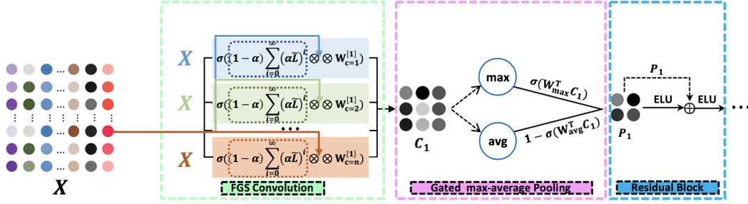
Fig. 1: Illustration Lévy Flights Graph Convolutional Network model. The input is the feature matrix  $X$  and the graph within dotted circle represents embedding Lévy Flights into random walks on graph (where  $L^\gamma$  is the Laplacian matrix  $L$  to a power  $\gamma$ ). LFGCN architecture consists of three main components: (i) FGS convolutional layer with parallel structure; (ii) *gated max-average pooling* layer; (iii) activation block for residual learning.
