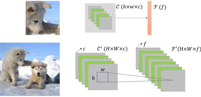
Fig. 7: **Fully-connected layer to convolutional layer**. Top: a patch-level fully-connected layer (in L2S-C<sup>2</sup>). Bottom: the corresponding image-level convolutional layer (in L2S-FCN).
