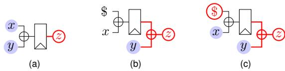
Fig. 3. Glitch-robust simulatability examples. Red circled variables are probes, thick red wires are glitches (probe extensions), blue background variables are inputs needed for simulation and the \$ sign denotes a random gate.
