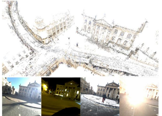
Fig. 1. Visual localization in changing urban conditions. We present three new datasets, *Aachen Day-Night*, *RobotCar Seasons* (shown) and *Extended CMU Seasons* for evaluating 6DOF localization against a prior 3D map (top) using registered query images taken from a wide variety of conditions (bottom), including day-night variation, weather, and seasonal changes over long periods of time.
