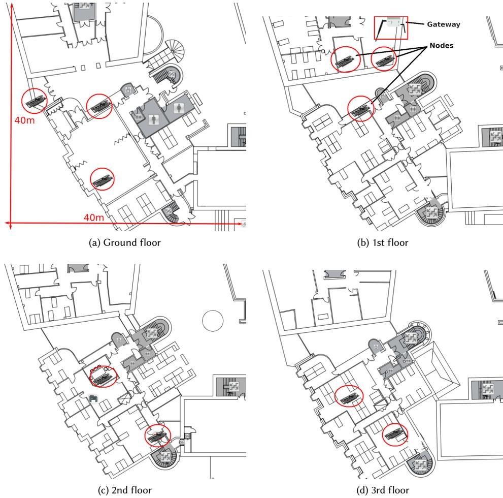
Fig. 7. Positions of the nodes and the gateway in the 4-floor building.
