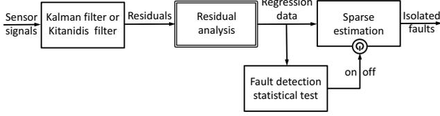
Fig. 1. Fault diagnosis flow chart. This paper is focused on residual analysis.
