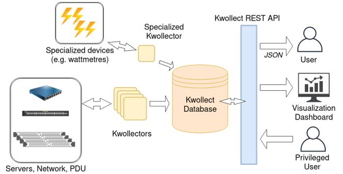
Fig. 1: Kwollect components
