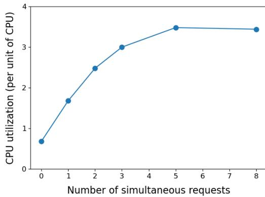
Fig. 7: Virtual machine CPU load as unit of CPU being busy (reported not being in the idle state by the *vmstat* tool), depending on the number of simultaneous user requests ongoing (average load over 60 seconds for each results)
