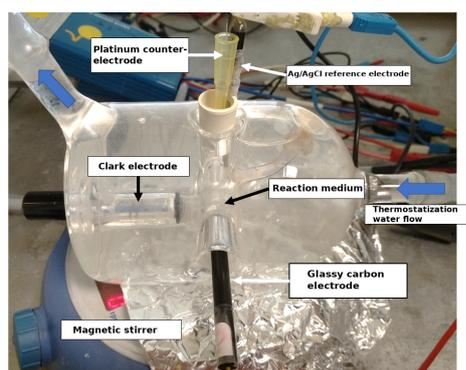
**Figure 4.** Oxygraphy chamber used to collect respiration data.
