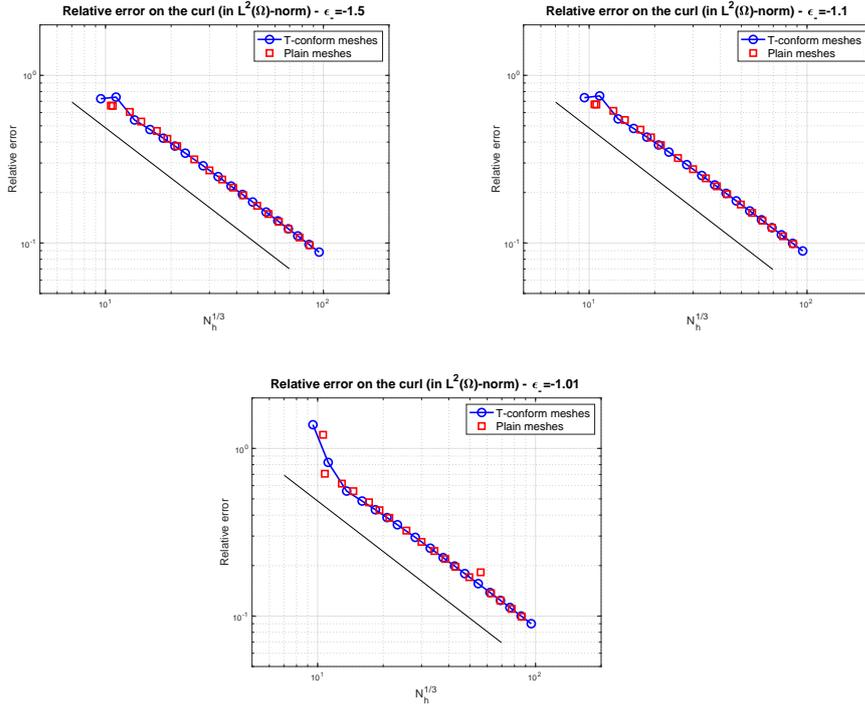
**Fig. 4** Relative error in  $L^2(\Omega)$ -norm of the curl obtained for the three values of  $\varepsilon_{|\Omega_-}$ , with  $h$  varying from 0.1 to 0.01. The line corresponds to the linear scale  $O(h) = O(N_h^{1/3})$ .
