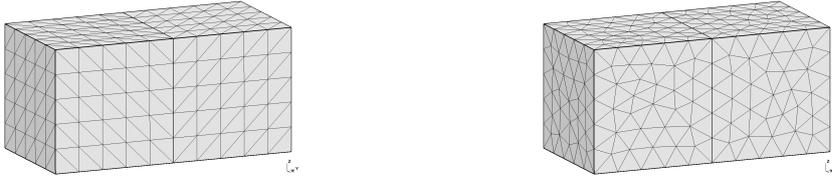
**Fig. 1** Left: a T-conform mesh; right: a plain mesh.
