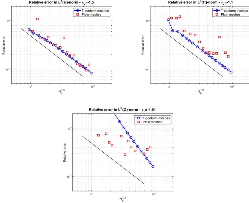
**Fig. 3** Relative error in  $L^2(\Omega)$ -norm obtained for the three values of  $\varepsilon|_{\Omega_-}$ , with  $h$  varying from 0.1 to 0.01. The line corresponds to the linear scale  $O(h) = O(N_h^{-1/3})$ .
