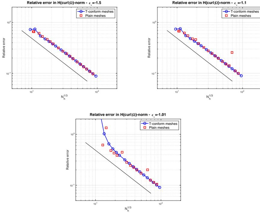
**Fig. 2** Relative error in  $\mathbf{H}(\text{curl};\Omega)$ -norm obtained for the three values of  $\varepsilon_{|\Omega_-}$ , with  $h$  varying from 0.1 to 0.01. The line corresponds to the linear scale  $O(h) = O(N_h^{-1/3})$ .
