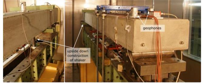
Figure 2. Concrete beam in the climate chamber.
