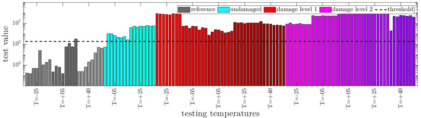
Figure 5. Test values at different testing temperatures in the undamaged state and at two damage levels. **Averaged** reference null space and covariance matrix are computed from a merged data set recorded at -25°C, 5°C, and 40°C.
