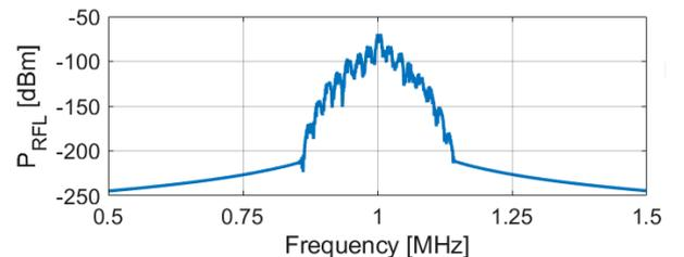
Fig. 5. Spectrum of the received RF signal when the local warning signal is predominant.
