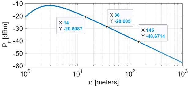
Fig. 3. Local FM signal's power variation with respect to the distance  $d$  between the car's aerial and the local FM emitter's antenna.
