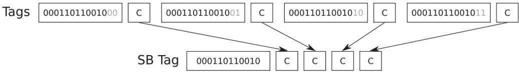
Fig. 3. Tag bits can be deduplicated if the tag field is reduced to accommodate only the **Most-significant Bits (MSB)** of the original tags. Since in this example there are four blocks per superblock, and the tag offset is only two-bits long, the differing tag bits can be stored implicitly through the order of the coherence fields.
