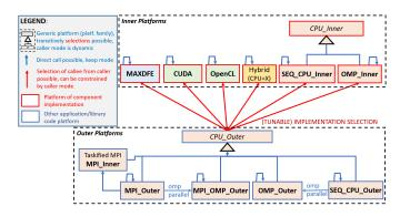
Fig. 2. The EXA2PRO "gearbox": Execution platforms/modes and implementation selection
