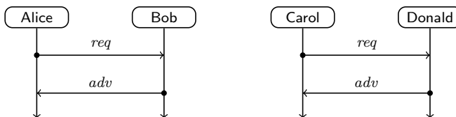
Figure 3: UML-like diagram of Systems 1 and 2 direct composition
