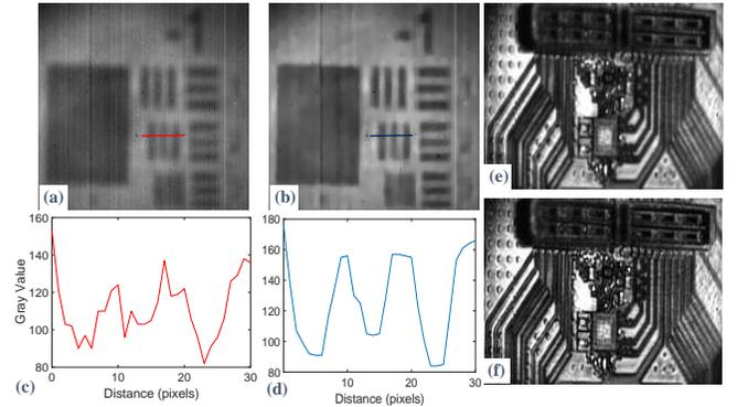
**Fig. 1.** (a) THz image of a 1951 USAF resolution test chart at 0.97 THz acquired with TZcam and x0.25 magnification lens. (b) Deconvolved image with  $\varphi_{-1}^{0.7}$ . (c) Plots of the Line Pairs pixel in grey values of the group-1 element 2 of the chart of original THz image, (d) deconvolved image. (e) Sample industrial application at 2.5THz. (f) Deconvolved image of (e) with  $\varphi_{-1}^1$ .
