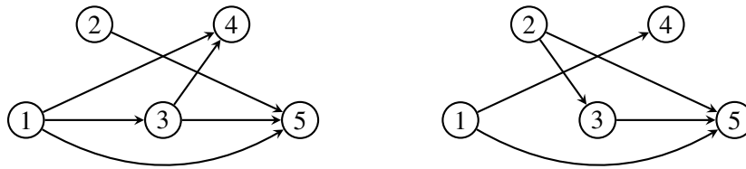
Figure 3: The dependency graphs for the two examples of Fig. 2; the left and right graphs correspond respectively to the single- and multi-agent examples presented therein. The active feedback at time t is exactly the set of in-neighbors of the corresponding vertex.
