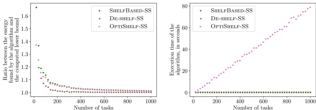
Figure 4: Output energy consumption and execution time to compute the solution for SHELFBASED-SS and optimizations (OPTISHELF and DE-SHELF) for instances with mixed power and Amdahl's tasks and  $p = 32$  processors (with  $P_{stat} = \frac{6}{155}$ ,  $\alpha = 3$ ,  $S = \{0.15, 0.4, 0.6, 0.8, 1\}$ ).
