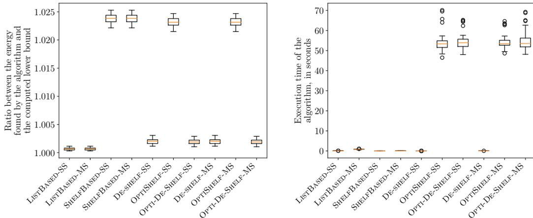
Figure 1: Output energy consumption and execution time to compute the solution for all ten heuristics with  $n = 500$  mixed power and Amdahl’s tasks and  $p = 32$  processors (with  $P_{stat} = \frac{6}{155}$ ,  $\alpha = 3$ ,  $S = \{0.15, 0.4, 0.6, 0.8, 1\}$ ).
