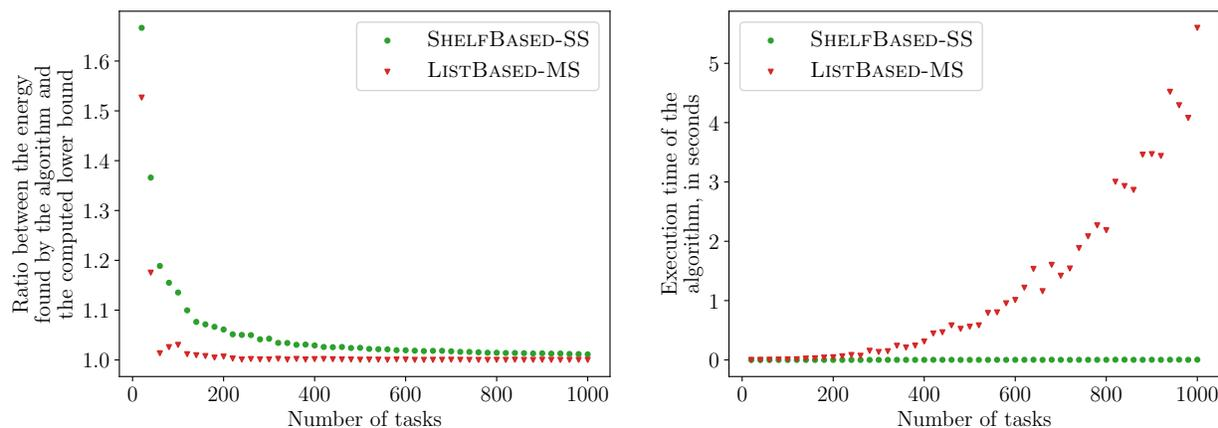
Figure 3: Output energy consumption and execution time to compute the solution for LISTBASED-MS and SHELFBASED-SS for instances with mixed power and Amdahl’s tasks and  $p = 32$  processors (with  $P_{stat} = \frac{6}{155}$ ,  $\alpha = 3$ ,  $S = \{0.15, 0.4, 0.6, 0.8, 1\}$ ).
