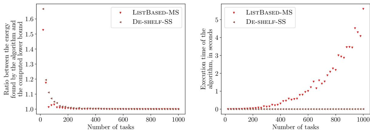
Figure 5: Output energy consumption and execution time to compute the solution for LISTBASED-MS and DE-SHELF-SS for instances with mixed power and Amdahl's tasks and  $p = 32$  processors (with  $P_{stat} = \frac{6}{155}$ ,  $\alpha = 3$ ,  $S = \{0.15, 0.4, 0.6, 0.8, 1\}$ ).
