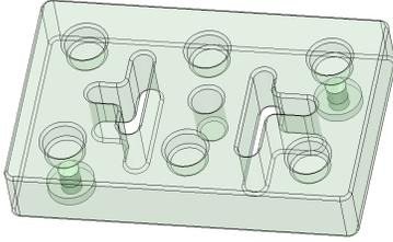
Fig. 3. EM model of the MDR filter.
