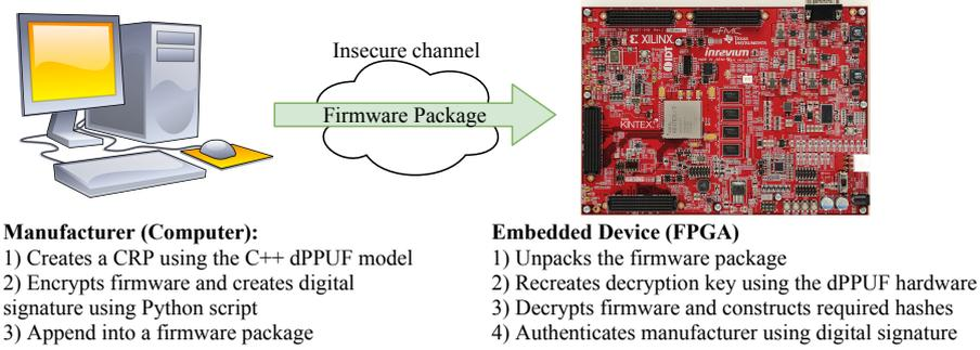
**Fig. 6.** Experimental and evaluation setup. The hardware-implemented security primitives are developed on a FPGA in order to emulate a dPPUF-enabled device. The firmware packaging procedure are carried out on a computer which is connected to the FPGA through a serial cable.
