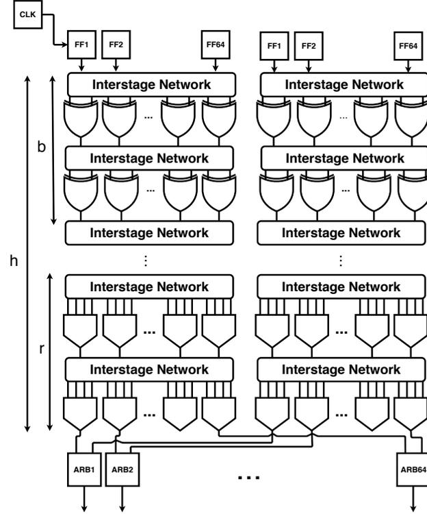
**Fig. 3.** The differential Public Physical Unclonable Function (dPPUF) architecture consists of consecutive layers of boosters and repressers. The two sides are identical in structure but different in inherent delays (inertial, propagation, switching, etc.). A layer of arbiters is placed at the end to capture the fastest propagating signals and according to the result, create the appropriate response bit string.
