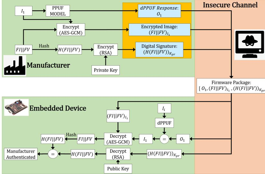
**Fig. 5.** The firmware package generation flow: the firmware vendor encrypts the composed image utilizing a public PUF model. The firmware unpacking process at the device level: the firmware package is decrypted, verified, and uploaded to the embedded device by utilizing public PUF’s (dPPUF) intrinsic manufacturing variability.
