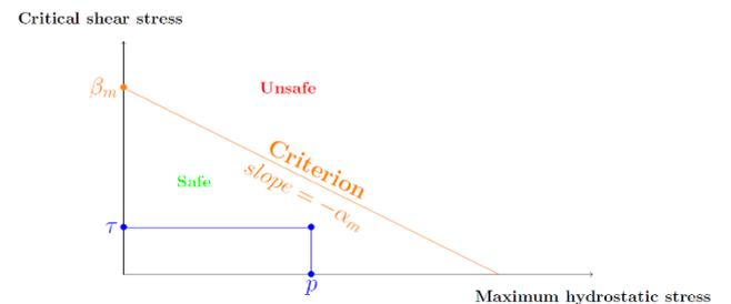
Figure 2: Dang Van criterion. A zone is safe (resp. unsafe) if  $(ph, \tau)$  below (resp. above) the straight line.
