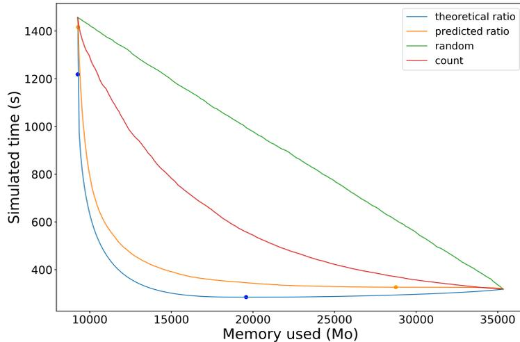
Figure 4: Simulated time of update tasks depending on the memory constraint for Geo1438 solved with a  $10^{-8}$  tolerance for four different heuristics. The training matrix for the predictive strategy is Serena using a  $10^{-8}$  tolerance. The top-left point represents the *Minimal Memory* strategy while the bottom-right point represents the *Just-In-Time* strategy.
