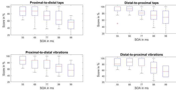
**Fig. 3.** Score when comparing five different SOAs vs. the reference one of 110 ms, across the two directions of motion (proximal-to-distal or distal-to-proximal) and type of stimulation (vibrations or taps). The boxplot gives the median, 25 and 75 percentiles with extrema values.
