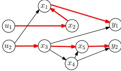
Fig. 2. Red edges represent an  $U$ - $Y$  linking of size 2 with minimum number of  $X$ -vertices, formed by the two paths  $(u_1, x_2), (x_2, x_1), (x_1, y_1)$ , and  $(u_2, x_3), (x_3, x_5), (x_5, y_2)$ .
