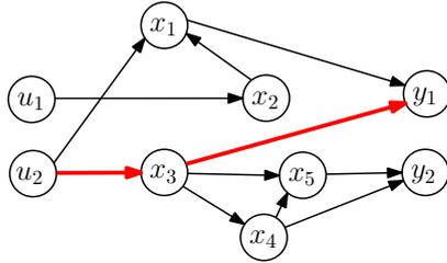
Fig. 3. Red edges represent an  $U$ - $Y$  linking of size 1 with minimum number of  $X$ -vertices: the path  $(u_2, x_3), (x_3, y_1)$ .
