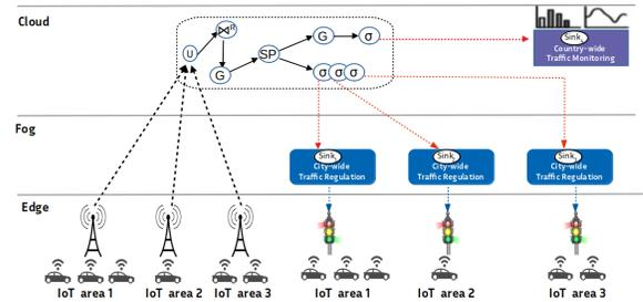
Fig. 1: Traffic management application adapted from [1]
