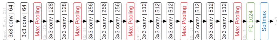
Fig. 6. Our model based on the VGG16 architecture.
