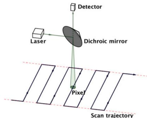
Fig. 1. Principle of a line scanning microscope
