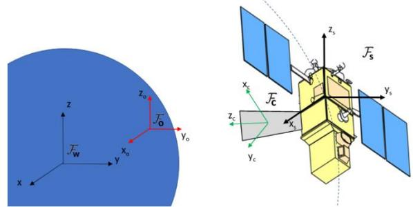
Figure 2: LION mission: a satellite ( $F_s$ ) directed by its orbital translation and controlled in rotation to track a terrestrial object of interest ( $F_o$ ) thanks to its camera ( $F_c$ ). World frame ( $F_w$ ) is here the equatorial geocentric frame of reference.
