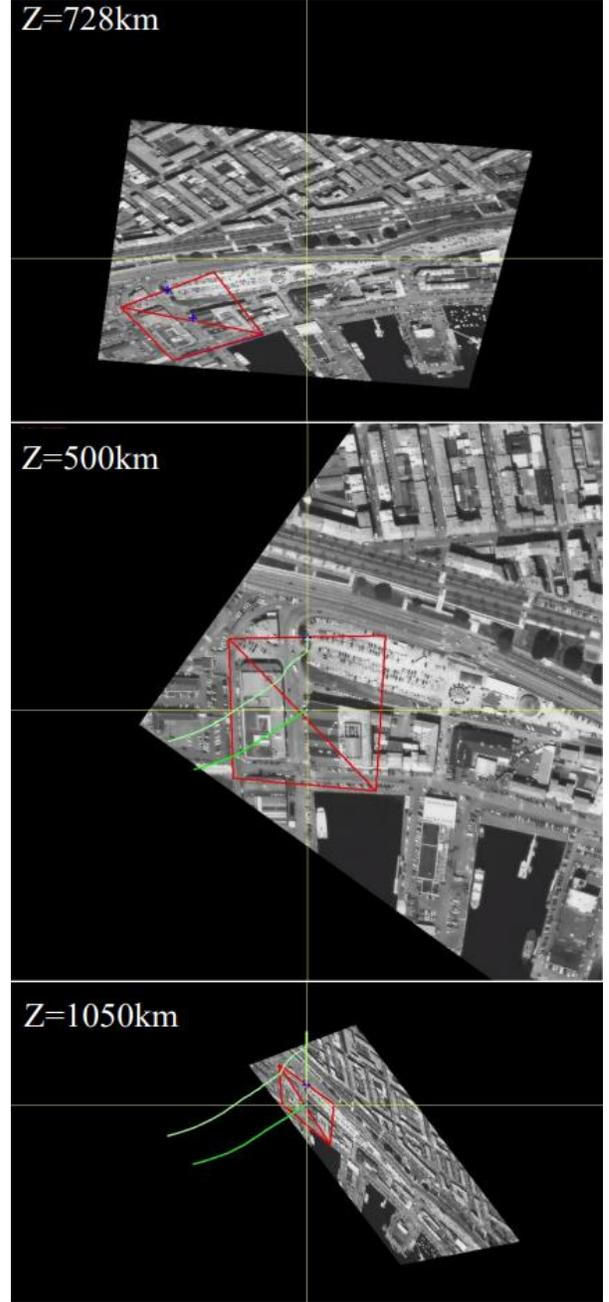
Figure 6: Image trajectory of point  $P$  and  $P'$  induced by visual control law in satellite simulation targeting an object of interest in the port of Brest. Satellite motion can be observed as it gets closer to the target, distance to target is reduced from 730km to 500km and both the image and the template are enlarged. After reaching zenith, the satellite moves away. The distance to target increases and the image and the template shrink.
