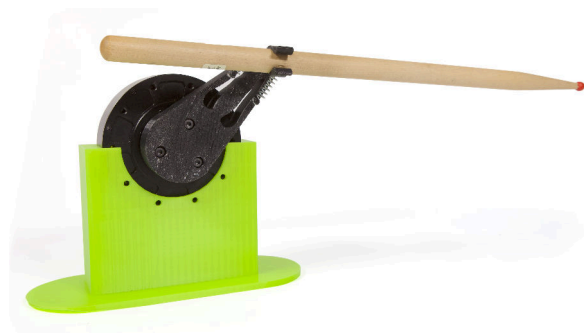
Figure 1: The robot prototype. The robot has two joints, one actuated by a servo motor and the other one contains passive springs to make the gripper flexible.
