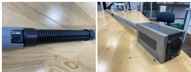
(a) Detail of spring and embedded microphone (b) Detail of box enclosure and speaker
