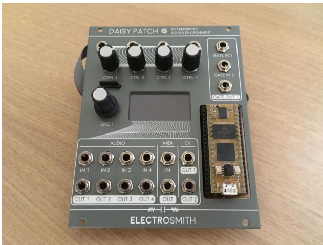
Figure 2: The Daisy Patch combines a predefined set of 4 knobs and linked CV inputs, 4 audio inputs and outputs, 2 CV outputs, 2 Gate inputs, 1 Gate output, 1 MIDI input and output, a rotary encoder, OLED screen and SD card reader. The Daisy Seed board can be seen on the lower right of the picture.
