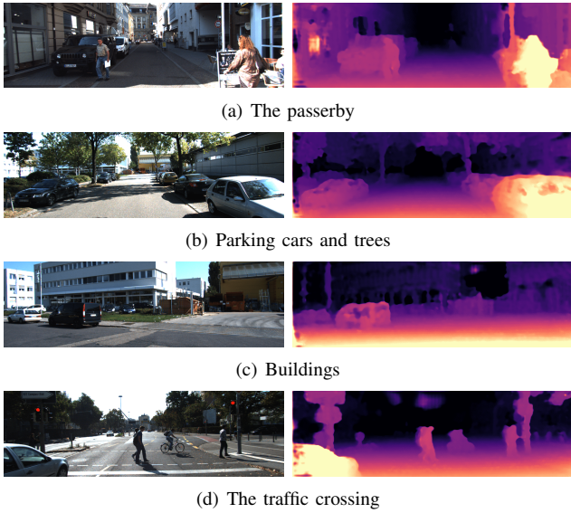
Fig. 2. Examples of depth maps from KITTI Depth test set (Eigen split).
