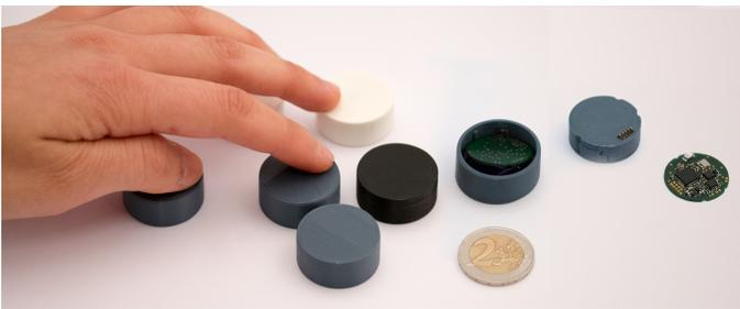
Based on the insights from our study, we created SmartTokens, tokens with embedded electronics that could sense how people touched, moved, and manipulated them. Each SmartToken included a 3D-printed cylinder, a custom circuit board, a small battery, six sensors for detecting touches, and a wireless transmitter for reporting inputs to a computer. The form factor of SmartTokens was chosen so that they could be easily grasped, and roughly five of them could fit comfortably in one hand.
