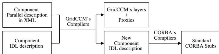
**Figure 5. Compilation steps to generate a parallel component.**
