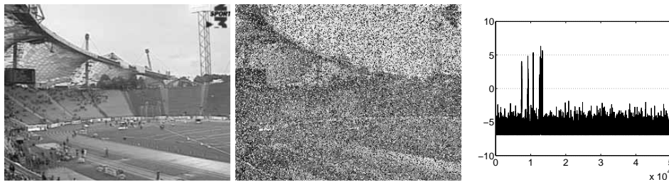
Figure 2: The middle image is a 50% impulse noise version of the original one. In a database of 10^5 images, they still match with a NFA close to 10^{-5} . The right plot shows -\log_{10}(NFA) for the first 50000 images of the sequence, the query being the noisy image. The peaks indeed correspond to exactly the same view of the stadium. The same views, but translated by 10 pixels, are not detected, since no prior registration has been performed.
