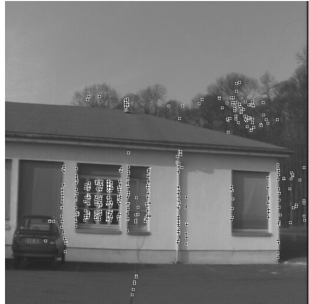
Fig. 6. Front view of flies evaluated with a fitness function using x component of Sobel gradient norms and a 5 \times 5 correlation window.
