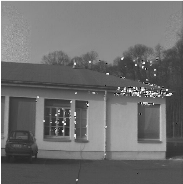
Fig. 4. Front view of flies evaluated with a fitness function using Sobel gradient norms and a 5 \times 5 correlation window.
