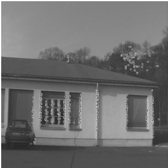
Fig. 9. Front view of flies evaluated with a fitness function using x component of Sobel gradient norms and a 23 \times 23 correlation window.
