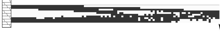
Figure 17: Optimal structure on the 100 \times 10 mesh for 10 \times 1 cantilever plate for the IFS representation. D_{lim} = 12 . weight = 0.58. CPU time = 15s/gen.
