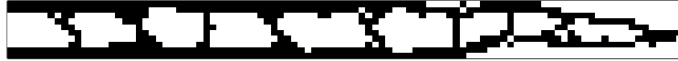
Figure 13: Optimal structure on the 100 \times 10 mesh for 10 \times 1 cantilever plate for the Voronoi-bar representation. D_{lim} = 12 , number of cells = 91. weight = 0.424. CPU time = 14s/gen.
