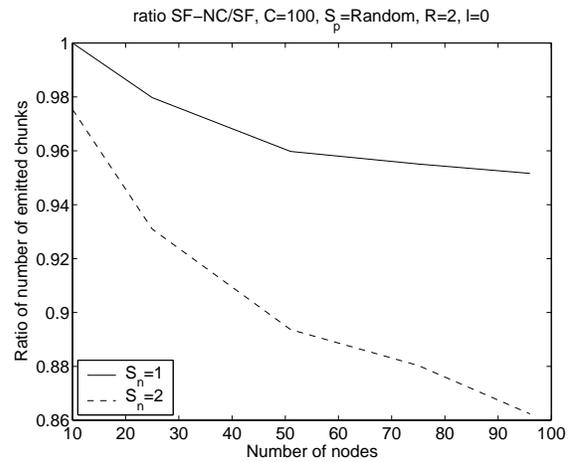
**Figure 4.** Ratio of the number of chunks emitted in *SF-NC* to *SF*. The number of chunks is  $|\mathcal{C}| = 100$  and the loss rate is  $\ell = 0$ . We consider two values for the number of sources  $S_n = \{1, 2\}$ .
