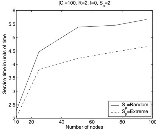
**Figure 5. Service time for  $SF-NC$  vs. number of nodes with two sources at two different placements  $S_p = \{Random, Extreme\}$ . We choose a number of chunks  $|C| = 100$  and a loss rate  $\ell = 0$ .**
