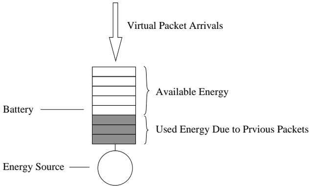
Fig. 1. The energy queue model: one queue case
