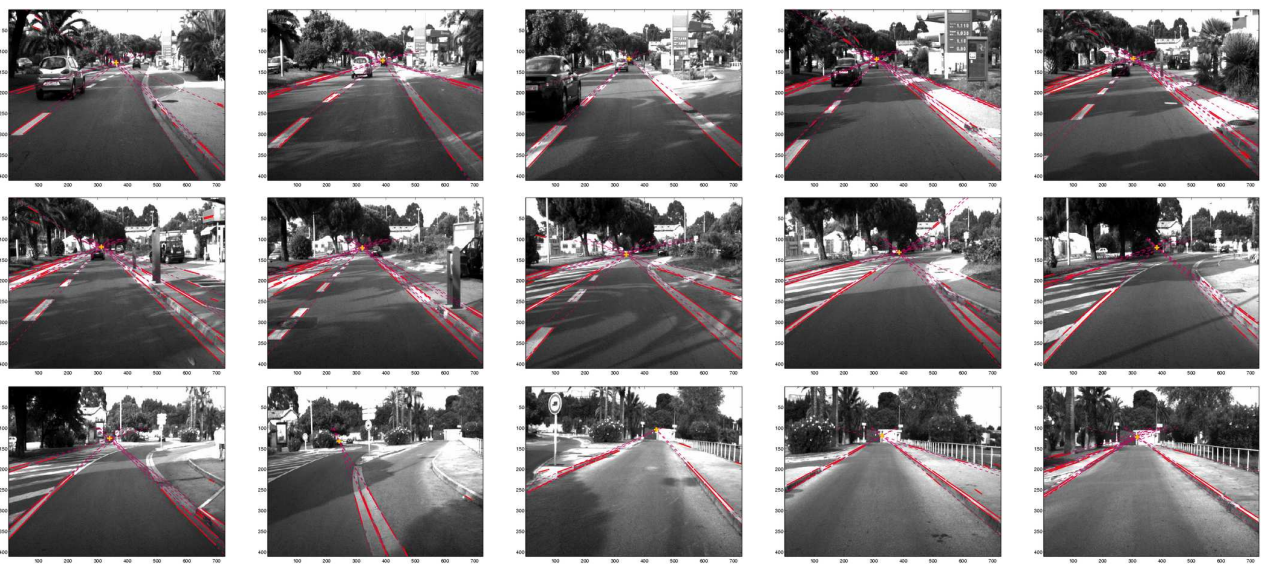
Fig. 5. Top-left, bottom-right, every 20 frames: results of continuous tracking of the DVP (orange '+') over a video sequence. The DVP is the weighted least square best estimation of intersection of all the VL candidates (red dashed lines).
