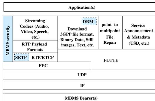
Figure 7: The MBMS protocol stack in the downlink.
