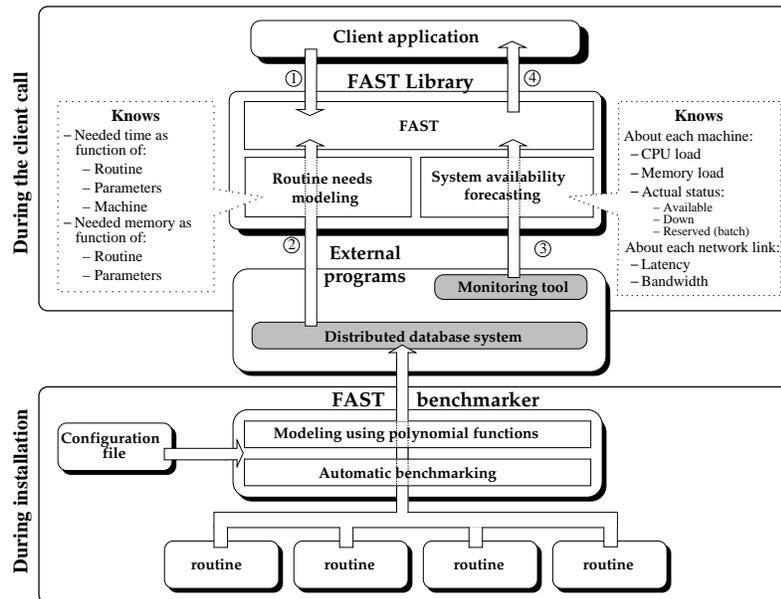
Figure 3: FAST's architecture.
